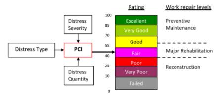
In 2018, the overall PCI rating at BFW was 42 (Fair). Several sample units in the 2018 inspection had a PCI rating in the 20s and 30s (Poor). Recent photos show further deterioration with large transverse cracks and significant infiltration of vegetation. Reconstruction of the runway is required.
